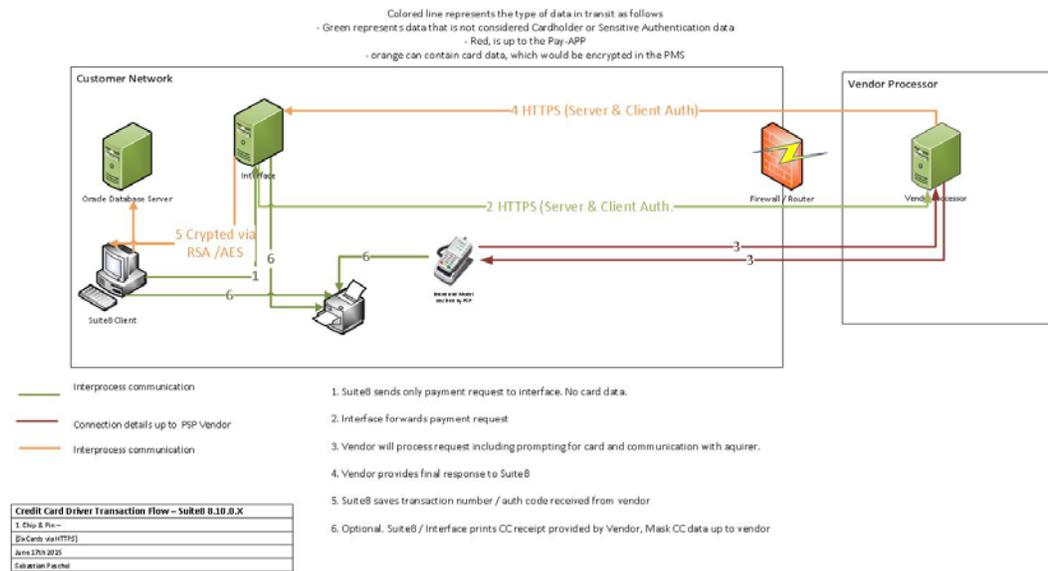
The following picture shows an example of the deployment diagram when a Chip & PIN interface is used:
