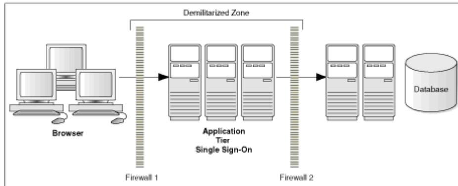
The term demilitarized zone (DMZ) refers to a server that is isolated by firewalls from both the Internet and the intranet, thus forming a buffer between the two. Firewalls separating DMZ zones provide two essential functions:
