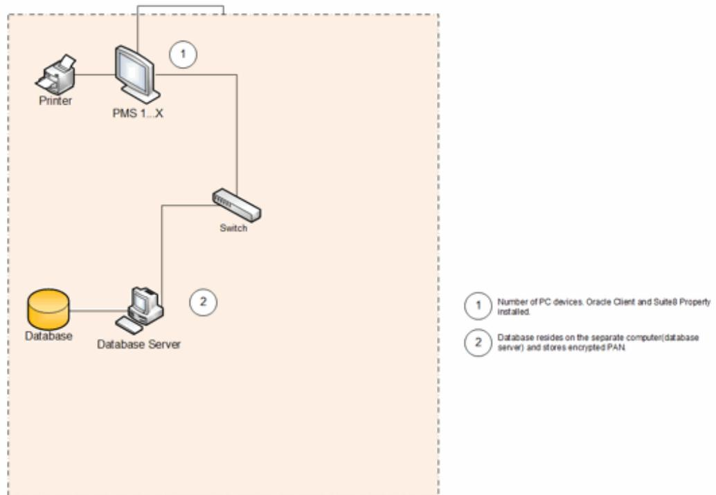
In accordance with the PA DSS Data Security Standard, Oracle strongly recommends that every site installs and maintains a firewall configuration to protect data. Configure your network so that databases and client PCs always reside behind a firewall and have no direct access to the Internet.
